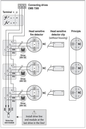
Line length and cross-section A (drives) depend on the type of drive and on the number of drives. Line length and cross-section can be determined according to the following formula:
