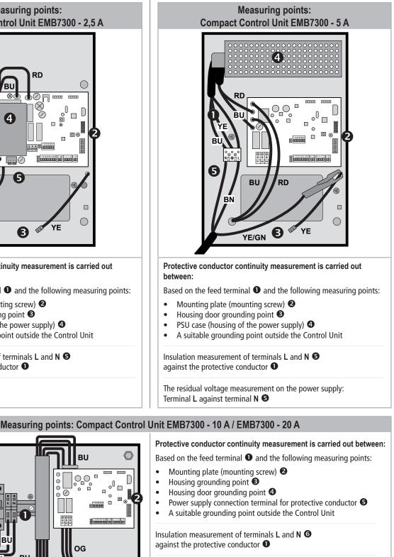
The residual voltage measurement on the power supply: Terminal L against terminal N 6
