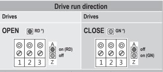
\*) The Duo-LED only lights up for the duration of the drive run time.
